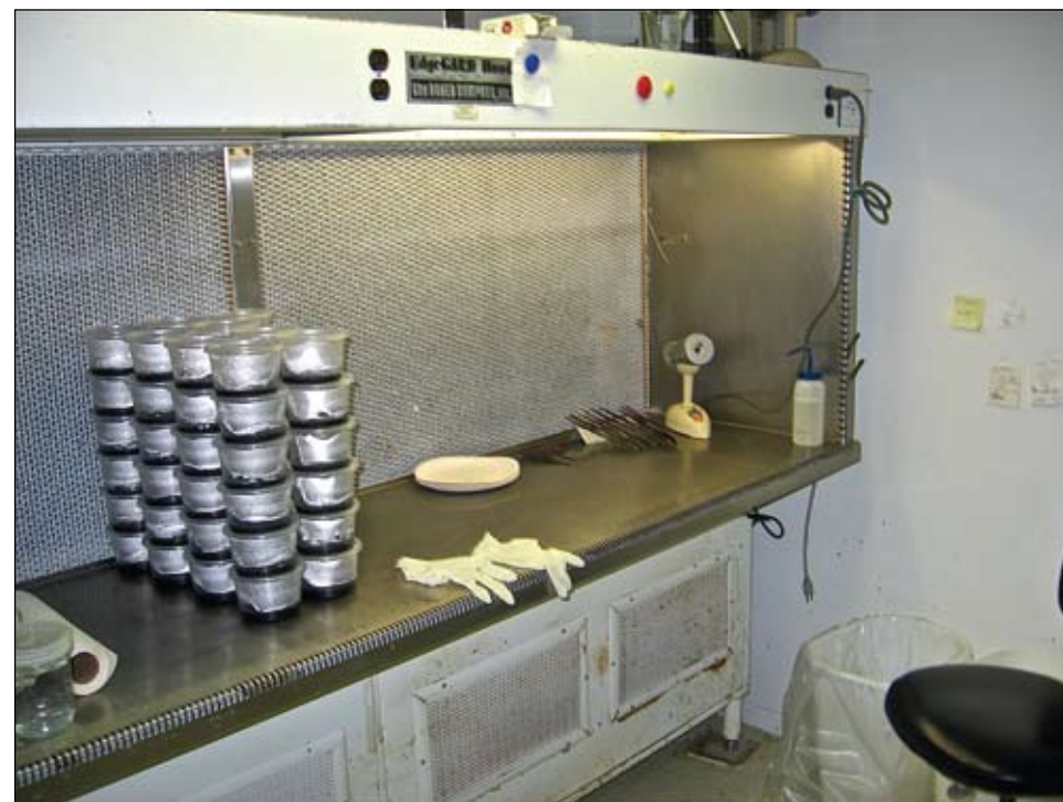
Figure 1. A "laminar flow cabinet" in the transfer room. Sterile air is blown over the bench to prevent contamination when sterilsed containers are opened.
